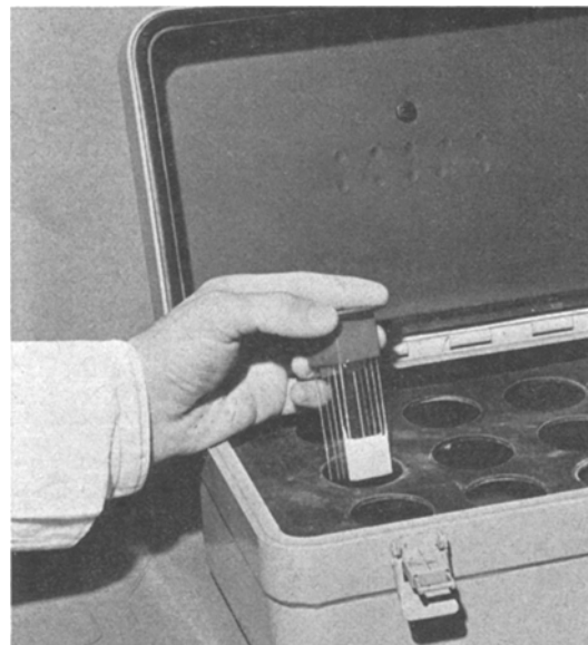
A Peel-A-Way slide holder containing 5 slides is being placed into a light-tight, air-tight box used for exposing radioautographs.
